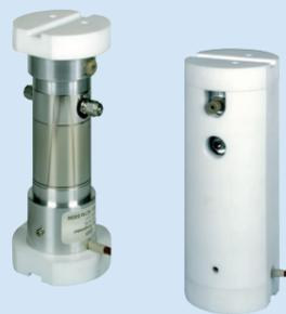
**HOVACAL** is based on the principle of dynamic evaporation of liquids and mixture with carrier gas. Liquid is continuously pumped into an electrically heated evaporator, vaporized and mixed with carrier gas. Liquid pump, flow controller for carrier gas and temperature controller are installed in the supply unit.
